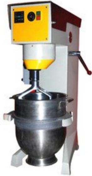
Tank made up of 2 mm. Stainless-Steel to withstand with the normal driving of Stirrer motor
