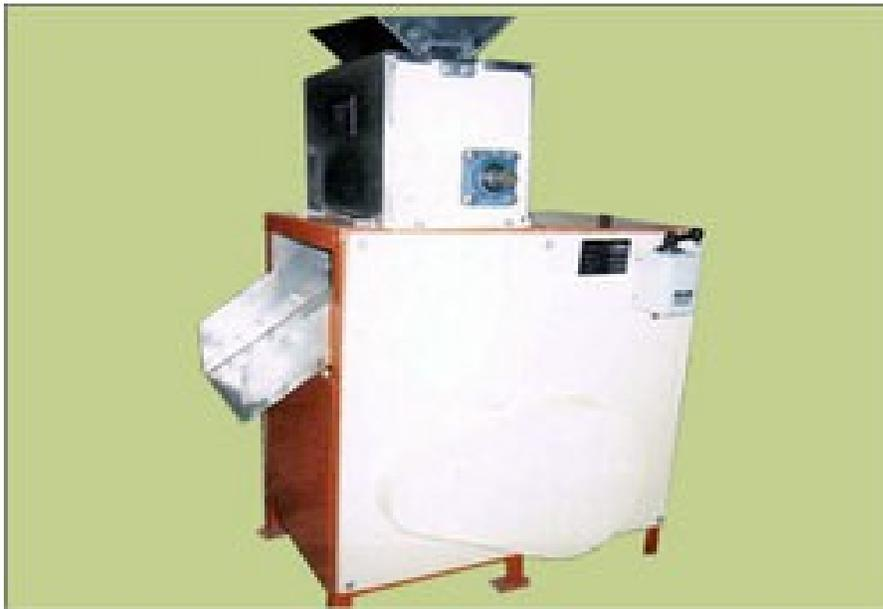
It is a proven mechanical system most commonly used for de Green Chilly cutting. All food contact parts and structure is made up of 304 Grade Stainless steel .Cut pieces are as per specifications or otherwise 20mm in length. Compact in size & easy for working. Long life SS Cutting blades. Feeding arm takes chilly through cutting blades.
