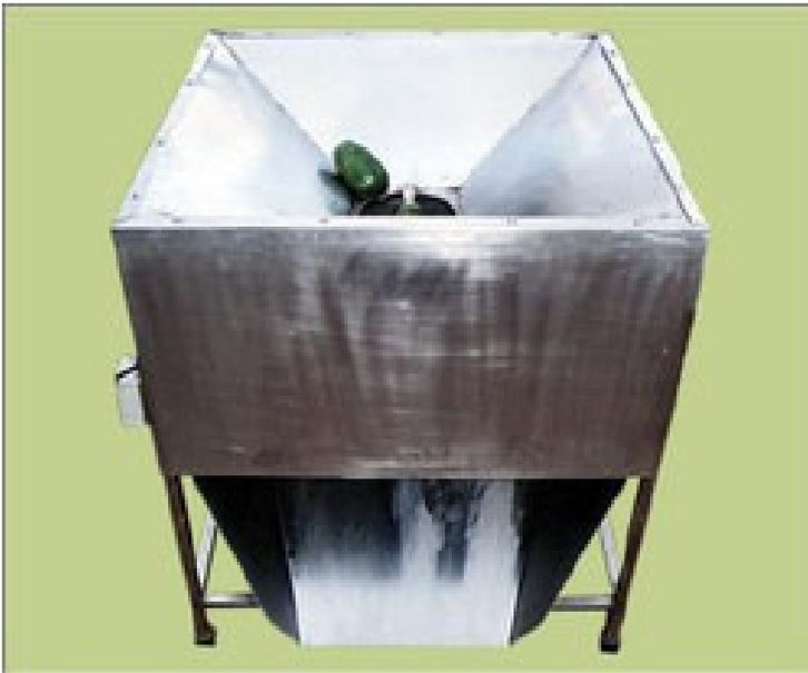
A complete SS 304 machine, mounted on anti vibration mounts, Structure of 3 mm formed sheet and other hoppers of 1.6 mm mat finish sheeting. Useful for FOUR PIECE cutting of Peeled Papayas before the de-seeding. Cutting is by 12" SS 410 cutters. Suitable for all regular sizes of Papayas and cutting collection in the mesh tray. Directly fed to multi purpose grader for de seeding about 90% cleaned papaya pieces. Feeding :Unload in Top tray. Easy to feed by hand.
