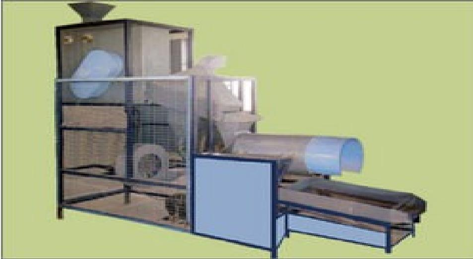
Useful for depotting and hard skin cleaning of garlic. M. S. Fabricated, duly spray-painted with provision of separation of garlic pots, dust, skin and dead pots separately, should be suitable to clean the maximum garlic of different season. (old garlic of 3 months minimum means at least naturally dried at once )
