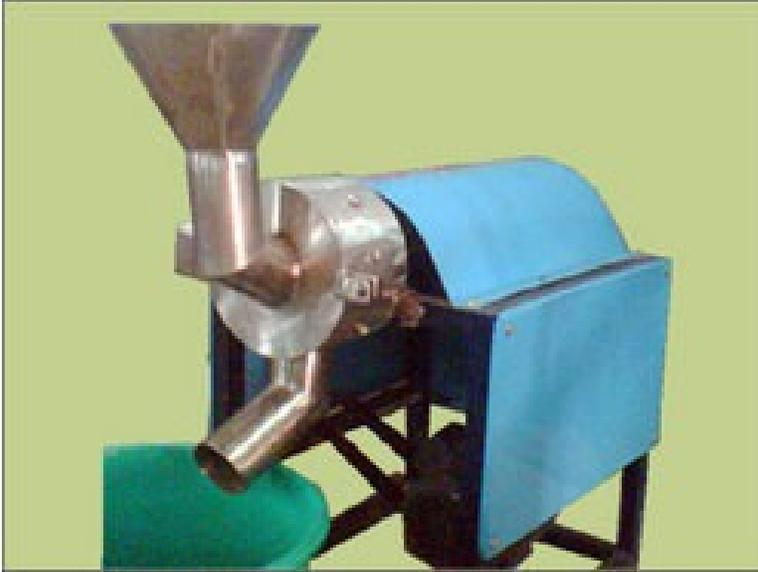
A proven mechanical system, all contact parts in S.S.304. It's most commonly used for Crushing of fruits into fine paste/ pieces for further operations. Useful for paste-making of Garlic-pods, hard material with body-fibres or shreads & for wet masala ingredients before mixing. Can be used for course paste, crush, mixes, multi-products crushing, Pre-crush for De-hydration inputs.
