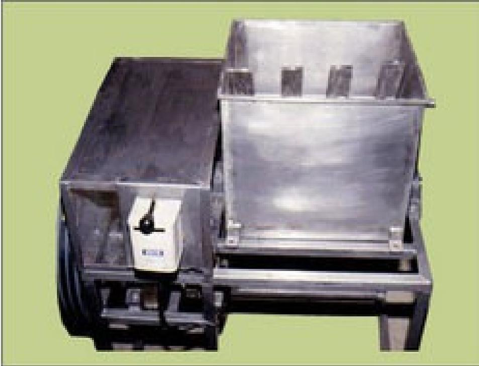
All food contact parts are made up of Stainless Steel with non stretching Rollers. Very useful the domestic production purpose. Foot operated machines gives you better out put and less manpower losses with minimum efforts. Pod of Dough is kept in two HDPE thick sheets and rolling is achieved.
